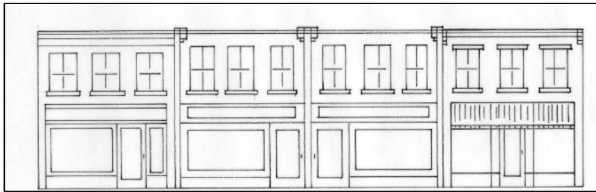
Figure 165 - New construction should be consistent with storefront and window size and spacing. In this sketch, the center two storefronts/buildings represent infill construction that mimic the rhythm and spacing of the adjacent historic storefronts
